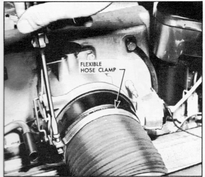
Fig. 29—Loosening Flexible Hose Clamp
